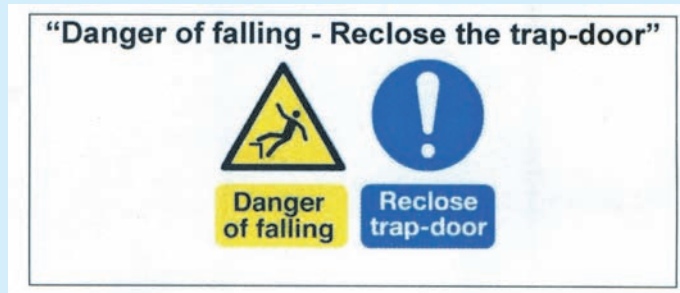
FIG. 5 TYPICAL NOTICE ON TRAP DOORS
