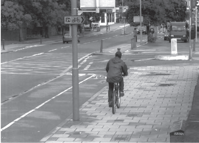
Fig. 27.4 Clock House, London. Poor design leads to poor discipline. A cyclist rides on the footway, whilst a pedestrian walks on the cycle track. Source: Tim Pharoah.
