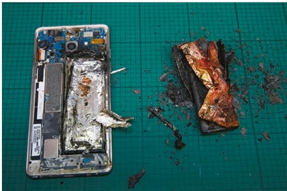
**Fig. 5.4** Battery explosion
