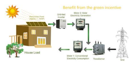
Fig. 11 Graphical representation of rooftop solar PV system [29]
