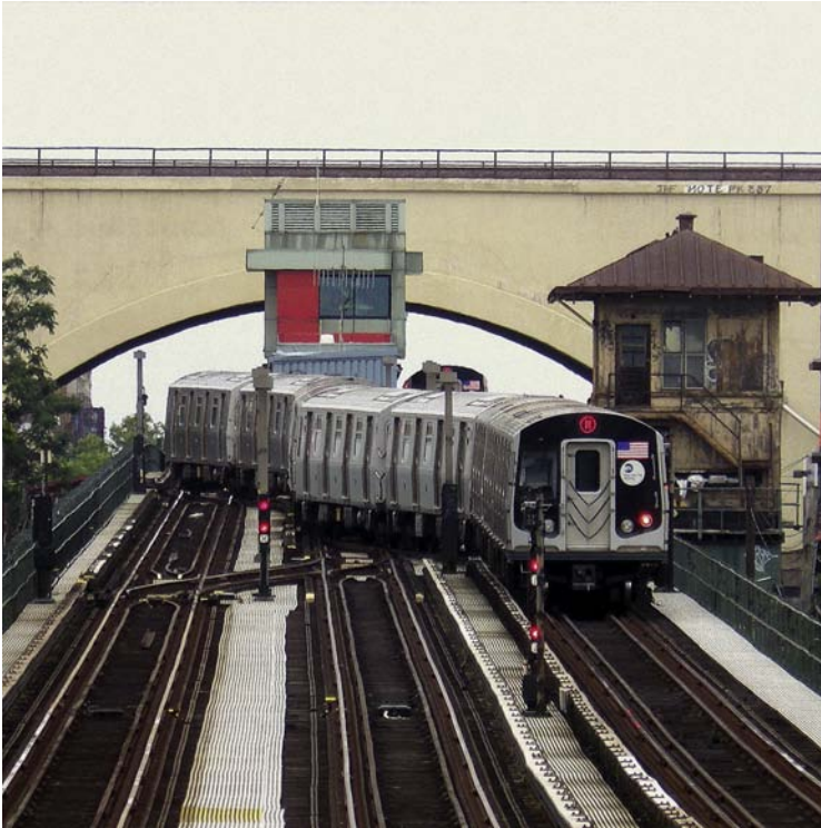
FIGURE C.18 N Train making cross over (switching from one track to another). Photo courtesy of Joe Raskin, http://wanderingnewyork.tumblr.com/ .
